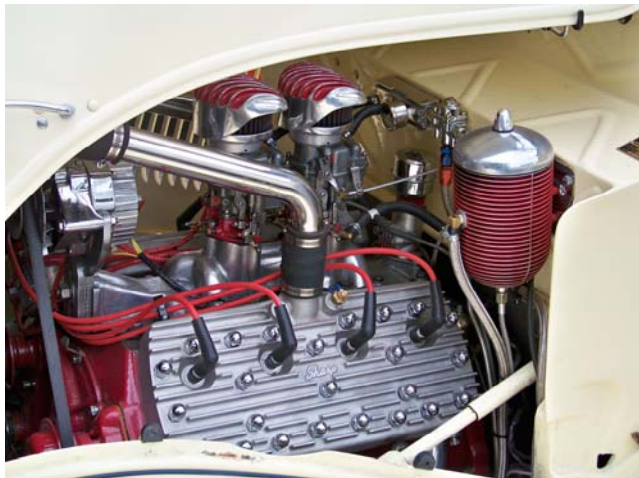
This 1933 Ford contained a period correct flathead equipped with Sharp cylinder heads—a common hot rod hop up item in the 1940's.
